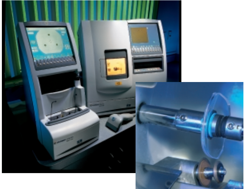
New, flexible soft cutting tool enables pin beveling on very thin, small diameter, and high minus or plus curved lenses.
